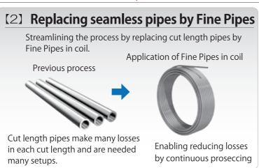
1) Replacing machined bars or (2) The secondary processing, such as seamless pipes by Fine Pipes tamping and pipe-end-sealing are also available, and outsourcing cost and managing cost will be reduced. (3) Fine pipes are provided in required length and increase productivity.
