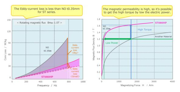
In automobiles, medical equipment and aerospace equipment market, various Compact• Highspeed Motors are used . Recently, the needs for High Efficiency rise even in these market. Nippon Kinzoku has developed the Electrical Steel Foils "ST080HP" to meet these needs. JAXA et al. has applied "ST080HP" to "Compact and High Efficiency Motors with the World's Best class High Power Density" by JAXA et al.
