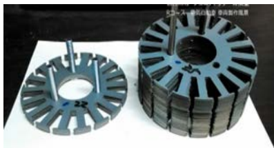
Non Grain Oriented Electrical Steel Foil, ST series “ST-150”
